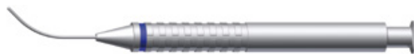
G-38631 SZURMAN DMEK IRRIGATION HANDPIECE curved, closed tip side port 0.3 mm tube 23 gauge / 0.6 mm
